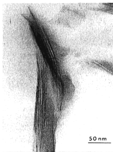
Figure 2. TEM images of the polystyrene nanocomposite of synthetic montmorillonite, SMM, derivatized with M2HTB.
