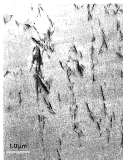
Figure 2. TEM images of the polystyrene nanocomposite of synthetic montmorillonite, SMM, derivatized with M2HTB.
